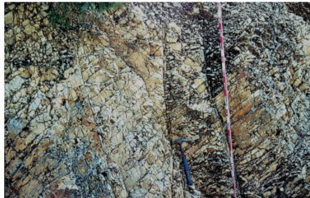
Ordovician quartzite. Poor quality. Weathered and heavily jointed rock mass.
